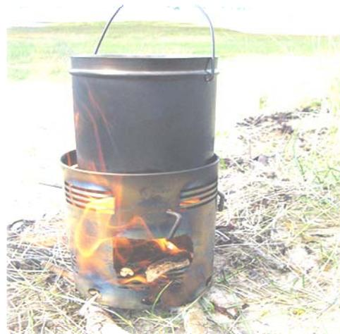
*The stove is typically made from an empty apple juice container; the Allen's Apple Juice is my personal preference. Simply cut out the bottom (and only the bottom as the top is your cooking surface), add vent holes to the top and cut an opening to add small sticks and twigs for fuel. The options for this stove are endless, get creative and have fun!*
